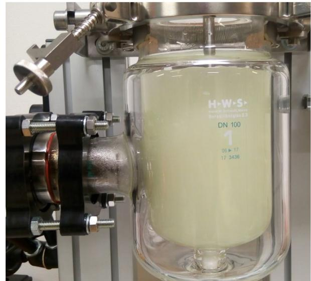
Figure 5. Droplet dispersion in a 1-liter laboratory reactor
