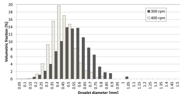
Figure 3. Droplet size distribution measured at two mixing speeds
