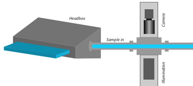
Figure 1. PFM installation in the process
