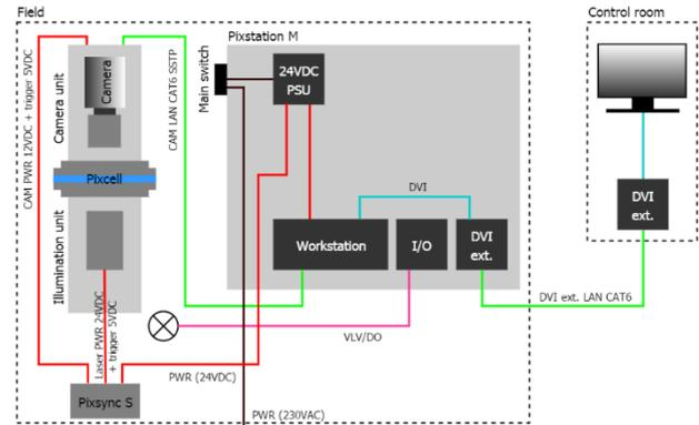
Figure 4. Connection diagram
