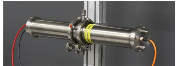
Figure 5. Pixcell flow-through cuvette with the illumination and camera units
