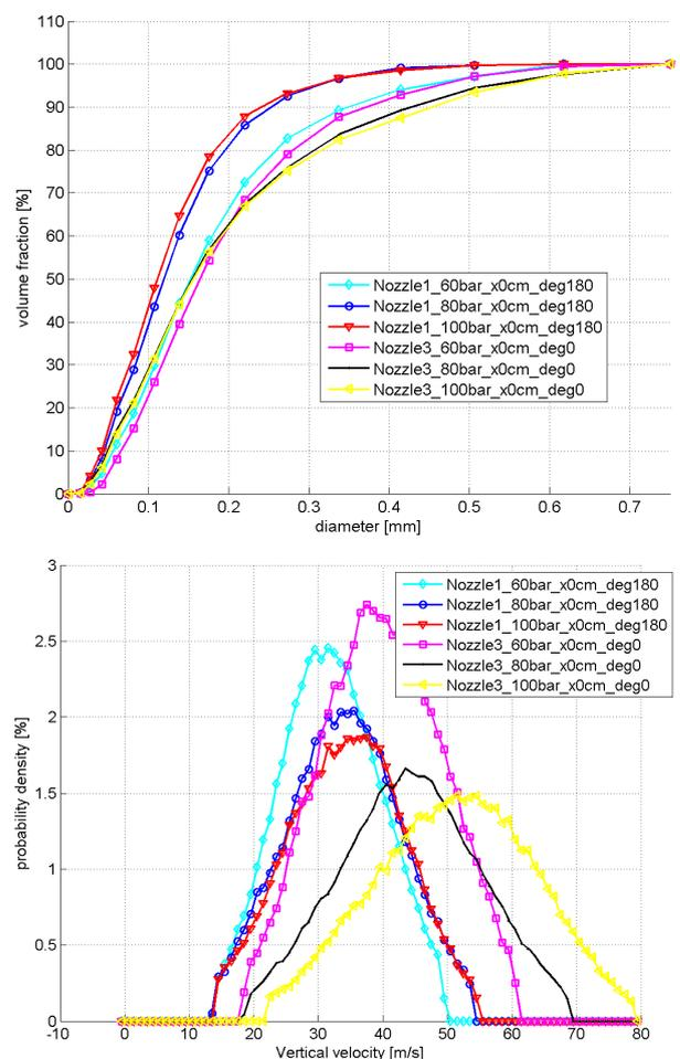
Figure 2. Comparison of droplet size and velocity distributions generated by two spray nozzles at three operating points
