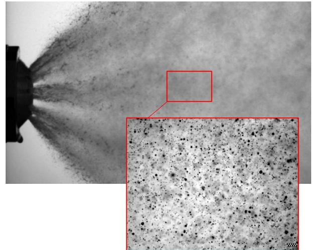
Figure 1. Examples of spray visualization and image data used for the droplet analysis
