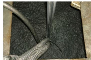
Figure 2. Imaging hardware submersed 1.5m beneath the froth layer of the mineral flotation cell
