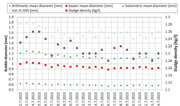
Figure 3. Bubble size and sludge density time trends
