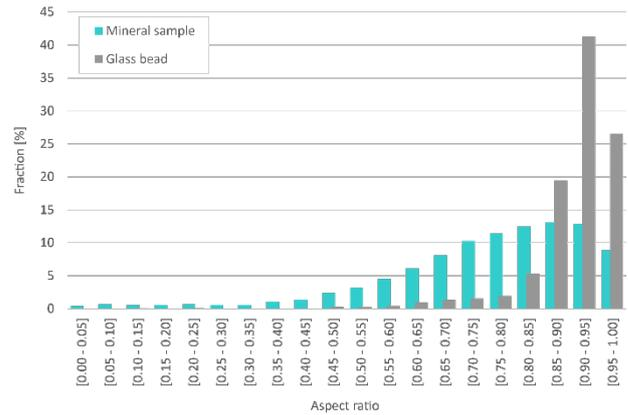
Figure 5. Particle aspect ratio distribution
