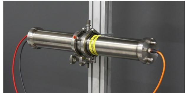
Figure 1. Pixcell flow-through cuvette
