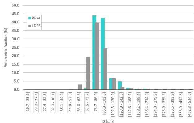
Figure 3. Volumetric size distributions for glass beads
