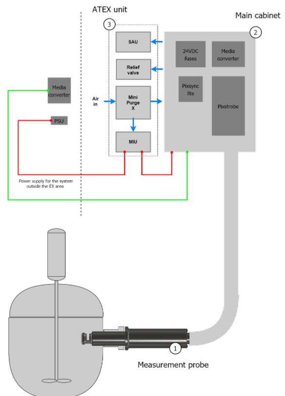
Figure 4. Layout and connection diagram of the measurement system
