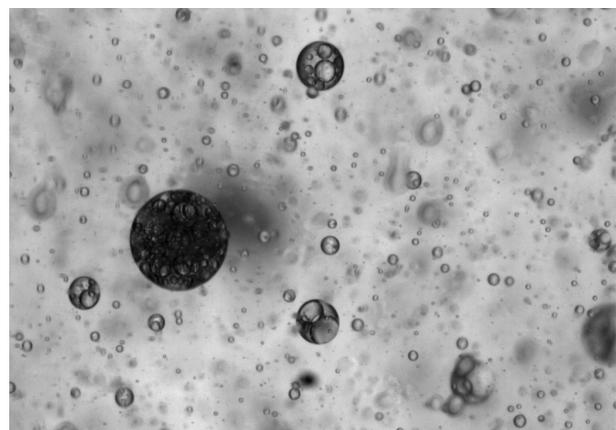
Figure 2. Droplets inside a droplet visualized by the PDM system
